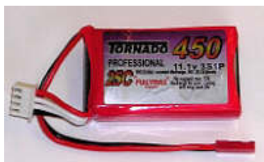
A 3-cell lithium polymer battery pack with balancing connector
